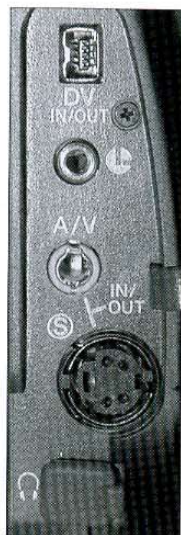
FIGURE 4.10 Be sure to determine what jacks your camera provides. This Canon GL-1 provides a headphone jack (bottom) on its rear panel, and a mini mic jack on a side panel (not shown).
